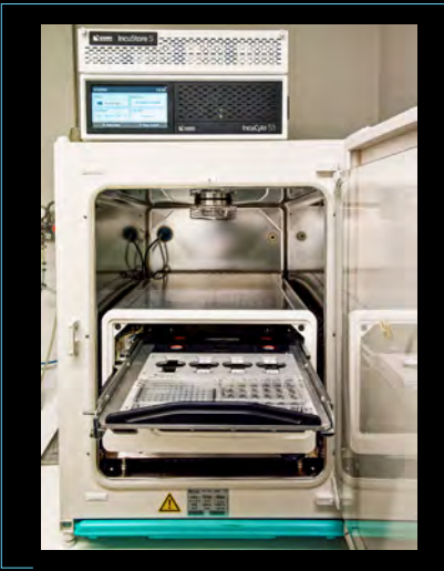
IncuCyte instrument inside an incubator, specifically designed for long term live cell imaging experiments.
