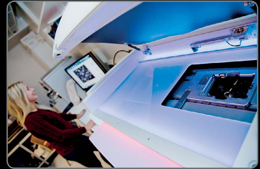
Perkin Elmer Operetta. A compact spinning disk confocal microscope, particularly designed for rapid analyses of fixed and live cells in microtiter plates.
